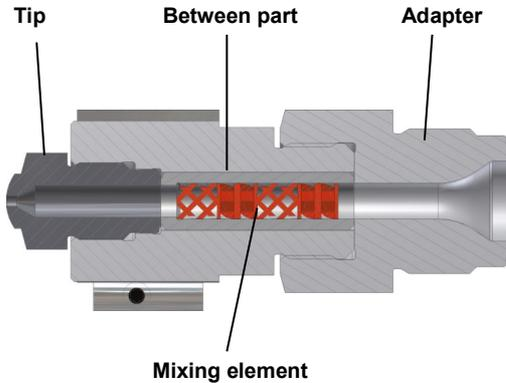
For the injection molding process a machine nozzle was developed, which is characterized by high mixing capacity with low pressure loss. The durable mixing elements are corrosion resistant and can be used also for abrasive media (until approx. 30% glass fiber portion).
